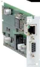
C = RS232+RJ (RS232 + Ethernet RJ-45 100 Mbs)
